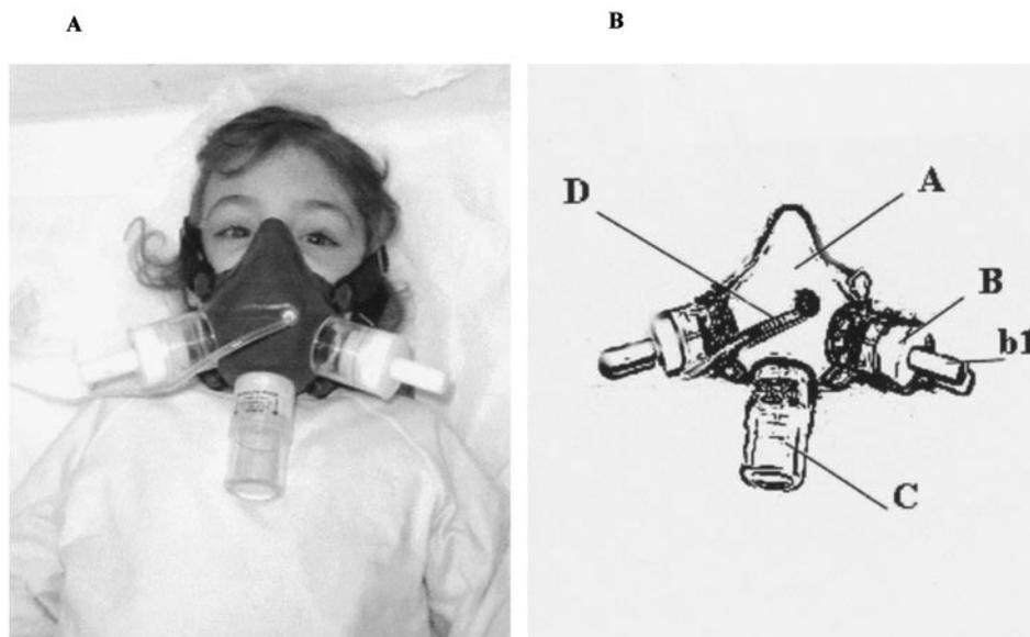
FIGURE 1. Left, panel A: Custom-designed nasal and mouth two-way, nonrebreathing facemask modified to simulate an inspiratory effort. Right, panel B: Facemask (A). The inhalation valve port (B) was adapted to lodge small plastic cylinders (b1). No extra respiratory resistance was applied to the expiratory port (C). The mask was also equipped with a transducer for measuring negative pressure generated by inspiratory efforts (D).
